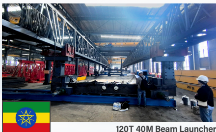
120T 40M Beam Launcher
